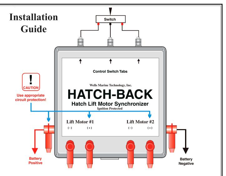
The Hatch Back is designed to control two worm gear motors used to lift heavy engine hatches simultaneously. The Hatch Back does this with very little current (approximately 1 amp) carried through the switch.
